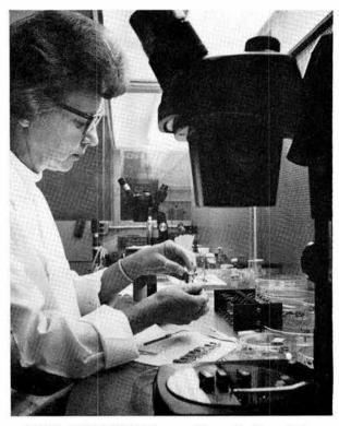
VERNA CLARK (4222-3) assembles rolamite switches at a clean bench location in the Rolamite Lab. A complete rolamite fabrication technology has been developed and transferred to oustide suppliers for production of rolamite switches.
